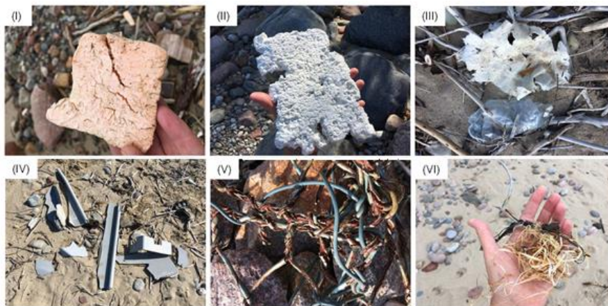
(I-II) various types of expanded polystyrene, (III) non-woven geotextile, (IV) facing fiberglass profiles, (V) gabion mesh with plastic coating (PVC / HDPE), (VI) fragments from a woven big bag (PP)
